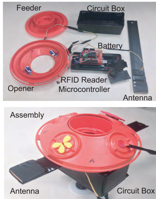
Figure 3. System assembly of the smart feeder. (Top) all components with the circuit box; (Bottom) final assembly.
